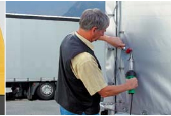
Repair welding of a truck tarpaulin using TRIAC PID with wide slot nozzle and pressure roller.
