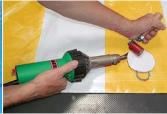
Welding tie downs with TRIAC S.
